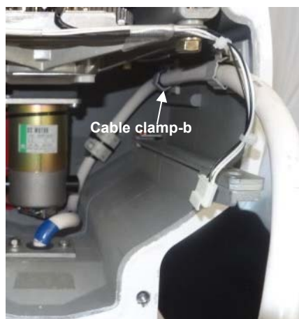
14) Clamp the cable by the cable clamp-b.
